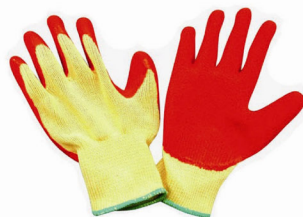
1362 Safety Glove * 10 Gauge Cotton, yellow dyed * Palm latex crinkle coated, Orange
