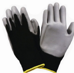
1391 Safety Glove * Palm Grey PU coated * 13 Gauge, Black Polyester lining
